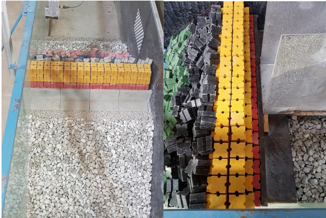
Figure 6.2: Regularly placed antifer units on the crest
