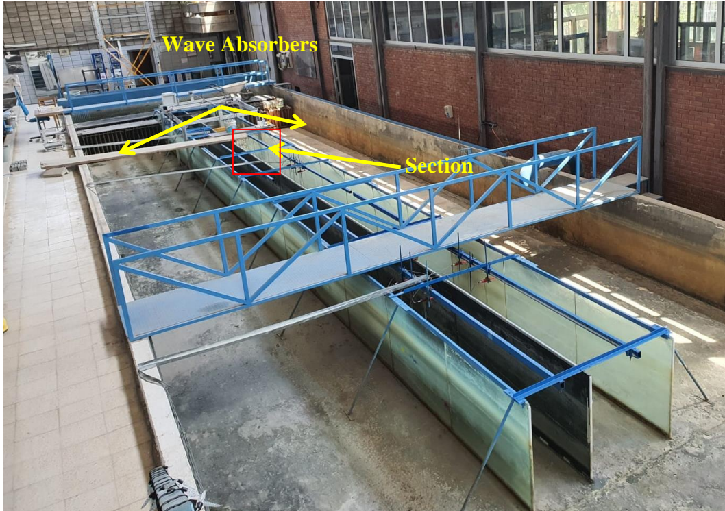
Figure 4.1: METU Civil Engineering Department, Coastal and Ocean Engineering Laboratory, Irregular Wave Channel.
