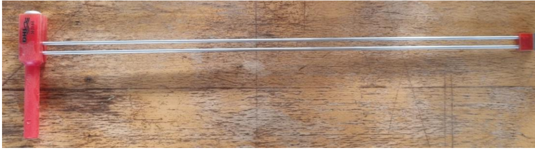
Figure 4.11: DHI-202 type 60 cm long wave gauge
