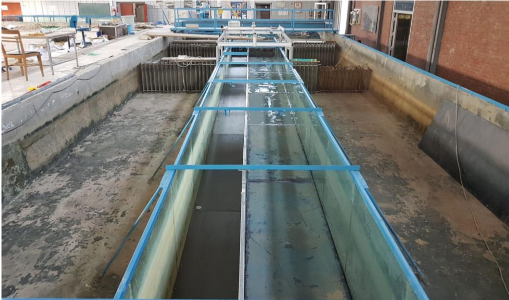
Figure 4.3: Wave channel and inner wave flume
