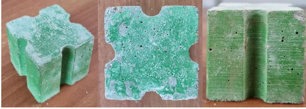
Figure 2.2: Oblique, plan, and cross-sectional views of anti-fer blocks used in the experiments
