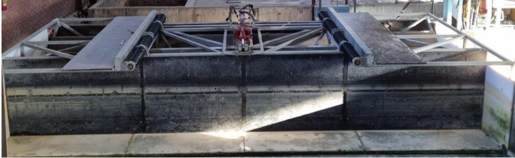
Figure 4.2: Piston type wave generator
