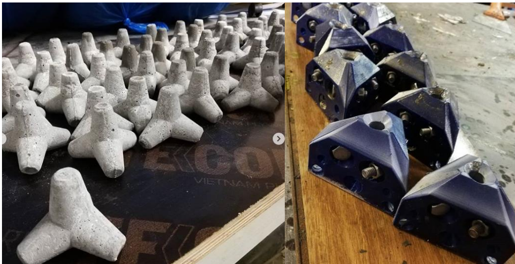
Figure 4.10: Example tetrapod units used in the experiments and their mold
